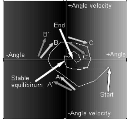
**Fig. 4b.** Actuator's behaviour with a permanent perturbation
