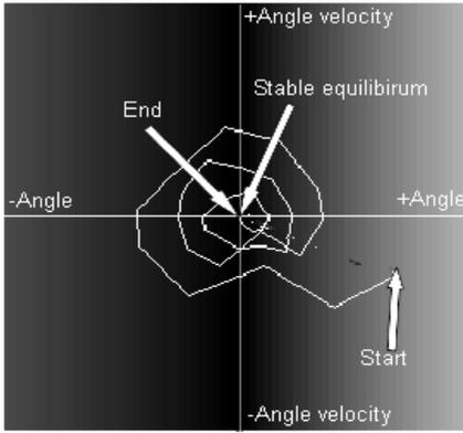
**Fig. 4a.** Actuator's behaviour without perturbation
