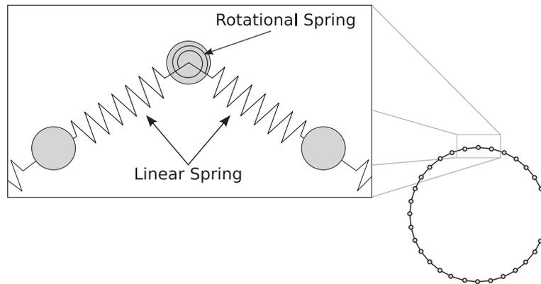
**Figure 3** Schematic of a membrane-section.
